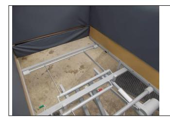
If there is a need to lower the foot section, the leg section limiter can be removed by dismantling the screws and lock nuts.
