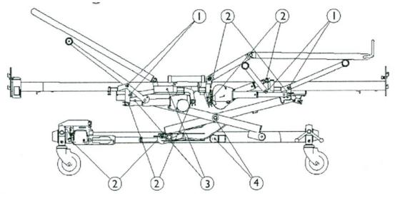
It is recommended to lubricate the bottom part of the HD Bed once a year according to the below plan:
